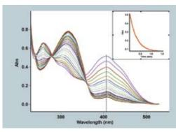
The Cary 50's extremely fast scan speed means that you can repetitively scan your kinetics sample many times during the reaction. Shown are 30 scans collected over 1 minute. The insert shows the kinetics curve at 410 nm.
