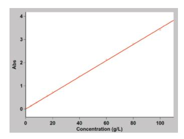
The Varian Cary 50's excellent linearity makes it ideal for measuring samples up to 3.5 Abs accurately and with confidence.
