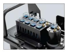
A range of automatic linear cell changers speeds and simplifies multi-sample measurements and quantitative calibrations.
