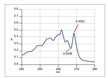
Figure 2. Pharmacopeia resolution test using 0.02% w/v toluene in hexane at 1 nm slit width. Ratio of peak and trough near 269 nm and 266 nm > 1.9 vs. the pass criterion of 1.5.
