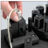
The temperature measurement kit provides precise in-cell temperature monitoring with real-time display within UV WinLab.
