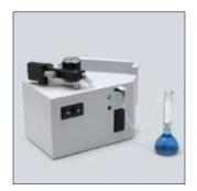
For liquids, the peristaltic sipper speeds throughput.
