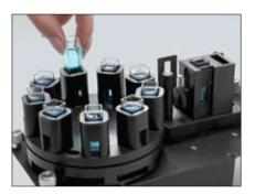
Peltier controllers accurately control the temperature of your experiment.
