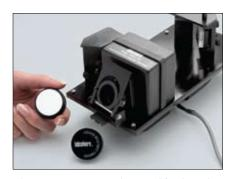
The sensitive integrating sphere simplifies the analysis of a wide variety of sample types, including solids, powders, pastes and liquids (LAMBDA 35 only).
